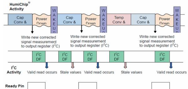
Figure 4.3.1: I<sup>2</sup>C Data Fetching in update mode
