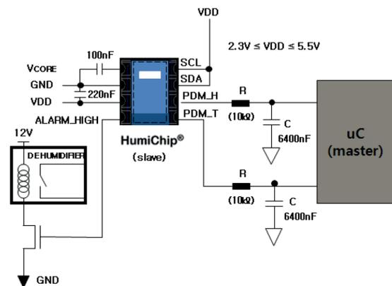
**Figure 6.1: Bang-Bang humidity control (high voltage application)**
