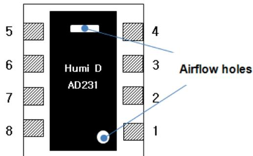
Figure 1.3: Laser marking
