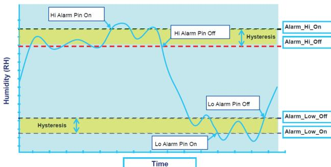
Figure 6.4: Example of alarm function
