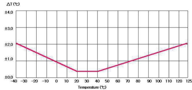
Abbildung 2: Typical Temperature Accuracy
