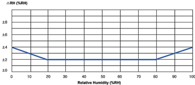
Abbildung 1: Typical RH% Accuracy at 25 °C
