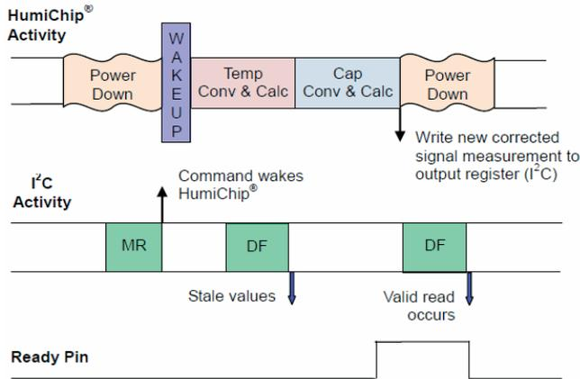
Figure 4.3.3: I<sup>2</sup>C Data Fetching in sleep mode
