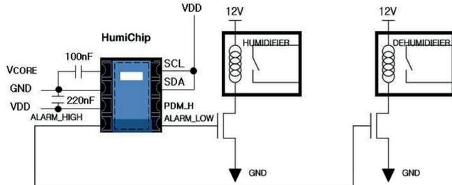
Figure 6.2: Bang-Bang humidity control (high voltage application)
