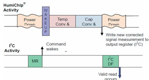
Figure 4.3.2: Measurement sequence in sleep mode
