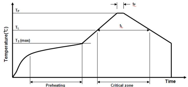
Figure 1.2: Soldering Profile (IPC/JEDEC Standard)
