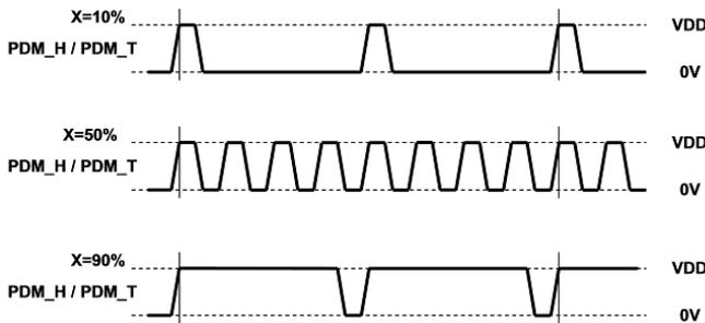
**Figure 5.1:** PDM signal timing diagram
