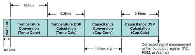
**Figure 4.1.3: Measurement cycle timing**
