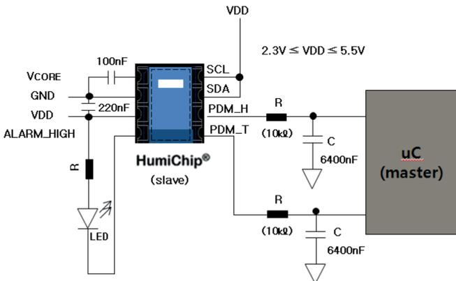
Figure 6.3: LED control with alarm function
