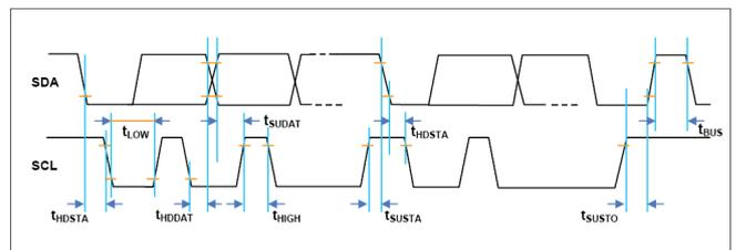
**Figure 4.2: I<sup>2</sup>C Timing diagram**
